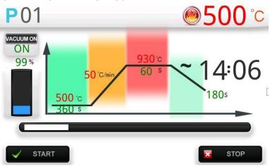
Press [Firing] in 1step firing interface, press [START] to start a 1 step firing program, the current firing program number which is the Program ID display number, pan will automatic down to the bottom, after ,you can put the porcelain teeth in the firing pan, It will automatically complete the firing process.
