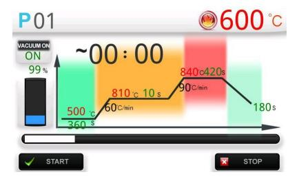
When the system is in **standby mode**, press **"2 STEP/GLAZE"** button to enter the **2 STEP** interface. At this time. After placing the glass, press **[start]** to start a **2 STEP** process. The **"VACUUM"** position shows the **VACUUM** status.
