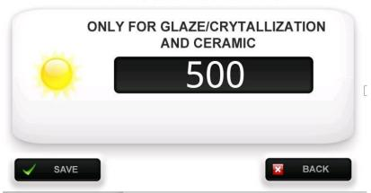
**Idle temperature** is Porcelain furnace not in firing ,a temperature value user hope to it static.
